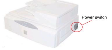
When you switch on the power, a yellow status LED on the control panel begins to flash. Wait until the scanner makes an audible "click" sound and the green status LED lights before turning on power to the PC.
